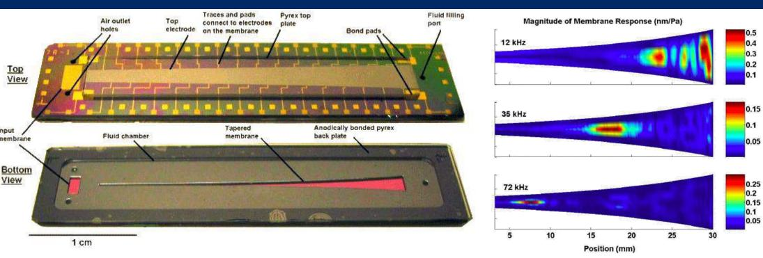
Understanding the mechanics of normal hearing is central to building prostheses and for improving noninvasive diagnostic tools. The Grosh Lab (Dept. of Mechanical Engineering works on various aspects of structural acoustics (the interaction of an elastic body with surrounding fluid), mechanics, biomechanics and linear/nonlinear vibrations. Pictured above is micromachined cochlear device developed for the purposes of designing better microphones and hydrophones.
