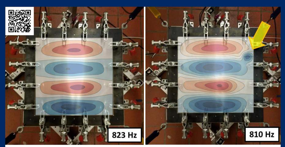
Laser Doppler Vibrometry measurements of a 12" square aluminum plate comparing resonances of a healthy plate (left) and a plate with a 1.5" cut (right). Vibro-acoustic changes are used for damage identification.
