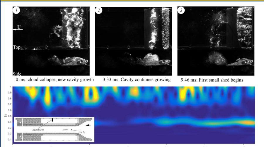
Steve Ceccio and his group (Naval Architecture and Marine Engineering) investigate multiphase flows using large-scale testing facilities. Of particular interest are cavitating flows from hydrodynamic surfaces. Shown above is the evolution of sheet cavitation behind a hydrofoil in a water tunnel. Acoustic measurements downstream are used to characterize the time-dependent cavitation dynamics.
